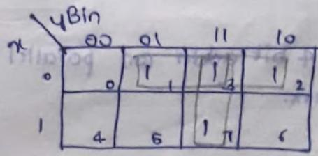
$$D = x\bar{y}\bar{B}_{in} + \bar{x}\bar{y}B_{in} + x\bar{y}B_{in} + \bar{x}y\bar{B}_{in}$$
