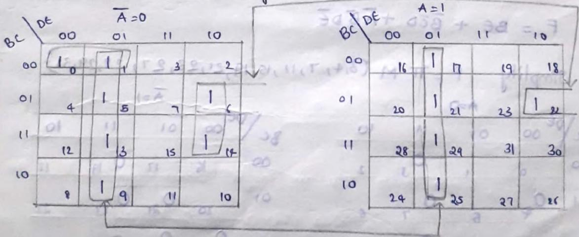
$F(A,B,C,D,E) = \bar{D}E + \bar{A}\bar{B}\bar{C}\bar{D} + \bar{A}CDE + \bar{B}CDE$
