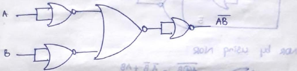
(5) EX-OR by using NOR :-  $A \oplus B = \bar{A}B + A\bar{B}$
