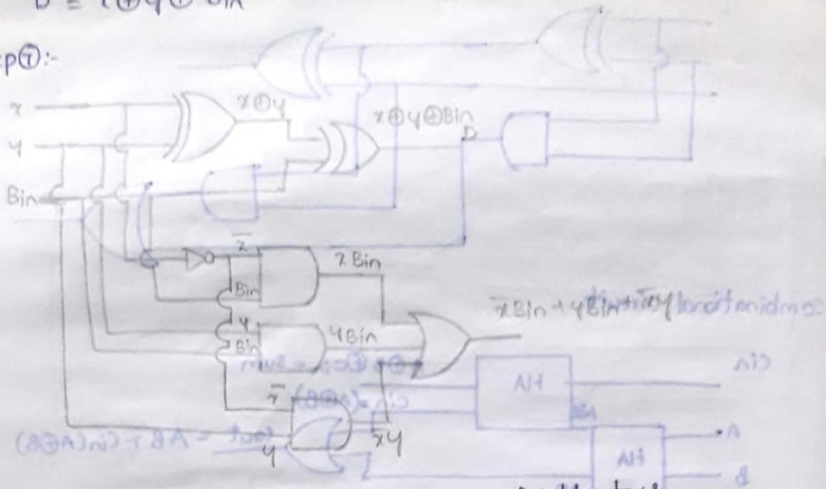
(9) Design full subtractor by using two half subtractor?
