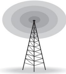
Fig: Omnidirectional antenna
