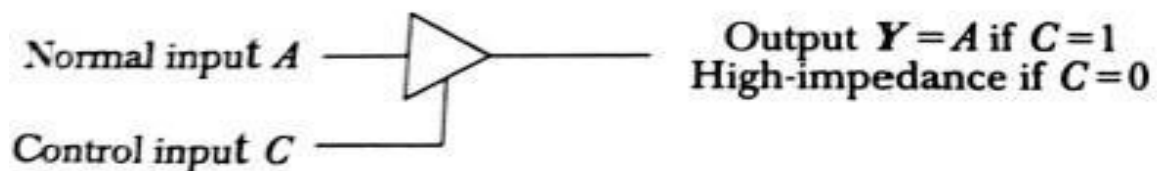
Figure 4-4 Graphic symbols for three-state buffer.
