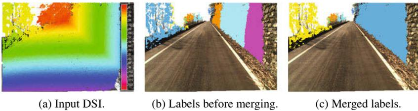
**Fig. 15** Obstacles labeling on a steep road when driving uphill. First points are clustered according to their relative pose, in parallel, on multiple CPU cores, then the labels are merged and filtered to produce the final obstacles list. Note that despite the slope the vehicle is facing, no false detection is triggered even without performing any explicit modeling of the ground.
